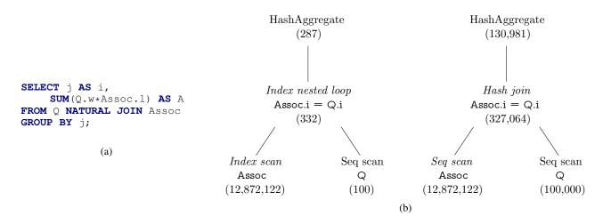
Figure 2: (a) Sample query. (b) Query plans for (a) given that Q is small (left) or large (right). Numbers in parentheses indicate table sizes. Italics indicate differences between the two plans.
