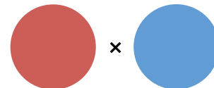
Figure 5. The landing pattern consisting of two colored discs (the cross identifies the target point that we use for landing).
