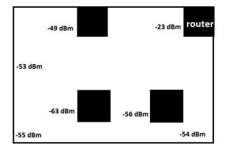
Figure 3: The signal strength was gathered from the outdoor environment. There was more signal attenuation, or loss in strength, behind the concrete obstacles.
