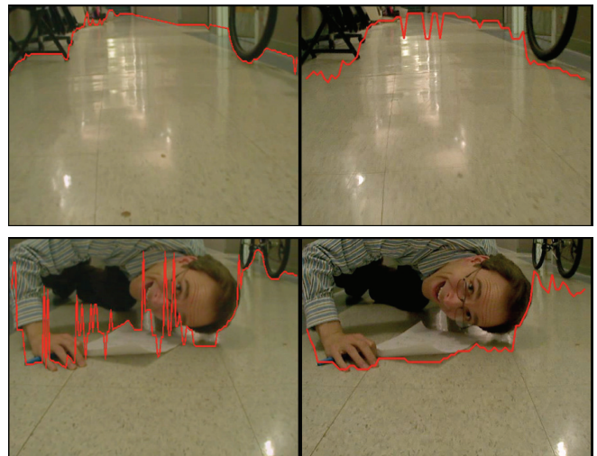
Figure 3. The results of our ground-plane segmentation based on both MLP and RBM networks. The images to the left in each case have been segmented by an MLP. Those on the right are segmented by an RBM. The greater precision of the MLP in familiar environments is evident in the top two images, whereas the greater ability of RBMs to generalize is apparent in the bottom two images: images containing a person did not appear in the training data.
