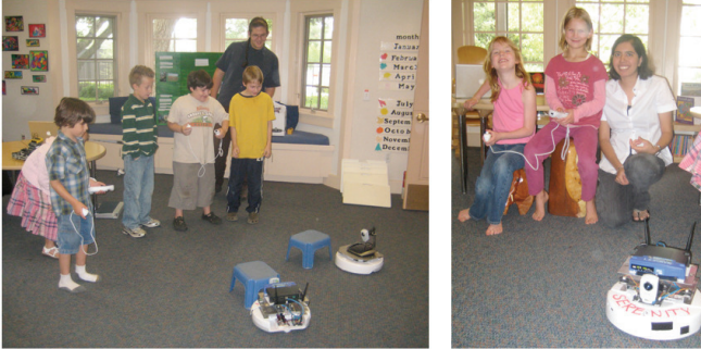
Figure 6. The resulting platform is seven-year-old-proof. Inexpensive enough to use in outreach activities, the software and Wiimote-control allows elementary school students to navigate the robots using only sensor-provided data.
