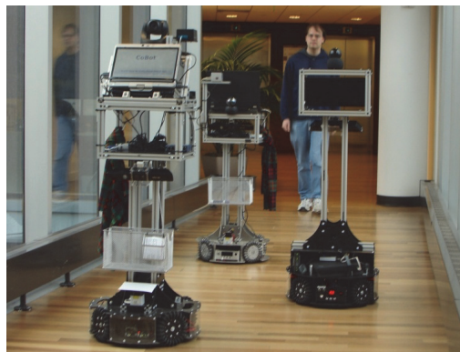
Figure 1: CoBot-1, CoBot-2 and CoBot-4 navigate through the building to deliver items requested by users.
