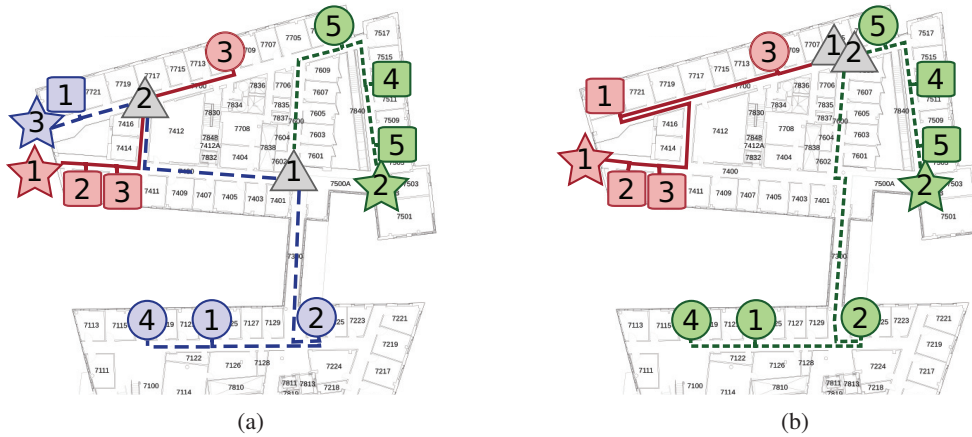
Figure 5: (a) Deliveries are scheduled with three robots (including two transfers). (b) When one of the robots dies and fails to respond, the tasks are rescheduled. See Fig. 2 for symbol meanings.
