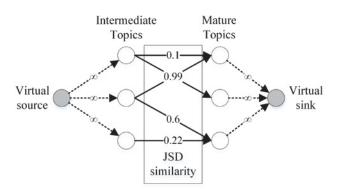
Figure 1. Bipartite graph depicting the potential matching based on JSD between topics, as well as the virtual source and sink used for the maximum flow algorithm.
