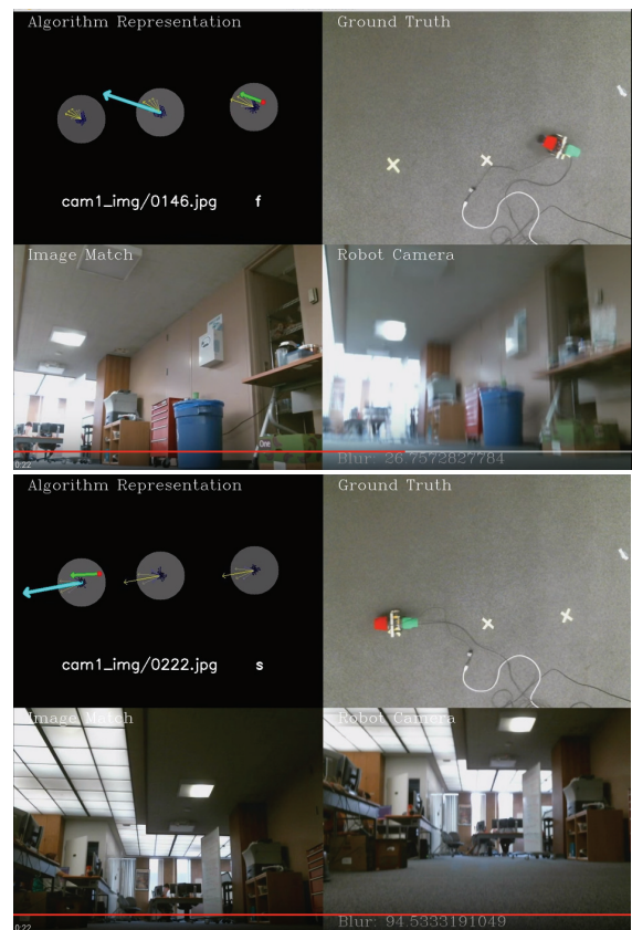
Figure 4. (Top) Snapshots from two different localization runs, each with three distinct map nodes and 24 distinct angles. By measuring and unweighting blurred images, the bottom run was more successful. (For additional detail, see text.)
