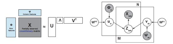
Figure 1: (Left) A high-level illustration of count/binary matrix factorization with side information given as features along rows and columns (the  $\approx$  is only meant to denote the underlying process). (Right) The graphical model for the proposed inductive non-negative latent factor model (hyperparameters not shown for brevity).
