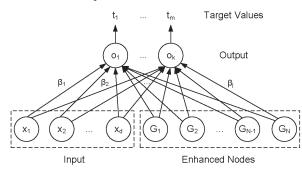
(b) Random vector functional link network (RVFL): d Input Nodes, N Random Neurons (equivalent to hidden nodes), k output Nodes.
