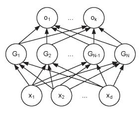
(a) Hidden Layer Neural Network: d Input Nodes, N hidden nodes, k output Nodes.
