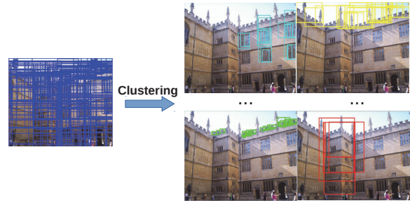
Figure 1: Hundreds of object proposals tend to overlap with each other. Through clustering, the object proposals containing the similar objects will be assigned to the same group.
