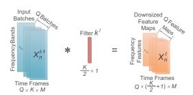
Figure 3: Convolution for frequency-dimension reduction.
