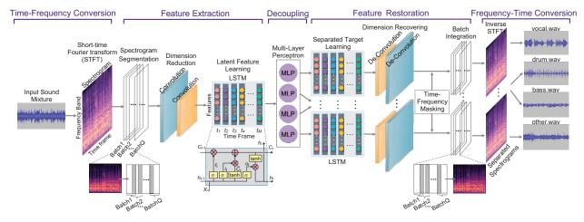
Figure 2: Illustration of architecture of Deep Representation-Decoupling Neural Networks (DRDNN).
