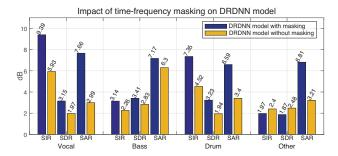
Figure 8: Impact of time-frequency masking.
