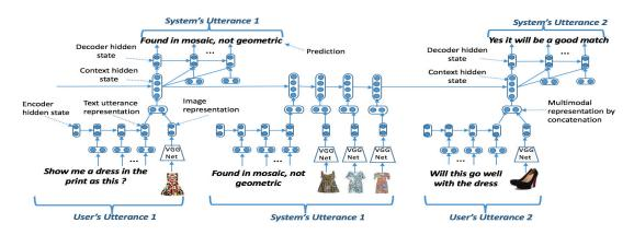
Figure 2: Multimodal Hierarchical Encoder Decoder Architecture for the Text Response Task. The figure shows all multimodal utterances, but in general utterances can have either modality or both.
