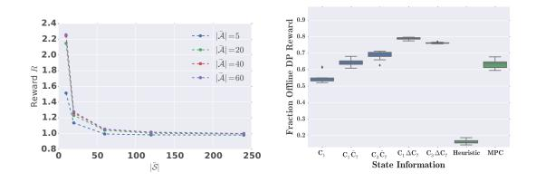
Figure 5: (Left, (a)) Optimal reward saturates for increasingly fine discretizations of our continuous MDP. (Right, (b)) HVFT - RL outperforms stochastic Model Predictive Control (MPC) and a heuristic relative to an upper bound oracle solution.
