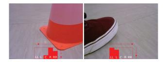
Figure 3: Camera view of the robot; outputs of the deployed net (red bars); resulting steering (horizontal slider) and linear speed (vertical slider).
