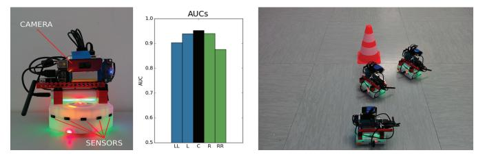
Figure 2: Left: custom Thymio used in this experiments, Center: performance of our neural network: AUC of binary predictions for each sensor (black - center, light blue - left, light green - right), Right: example of the robot's behavior
