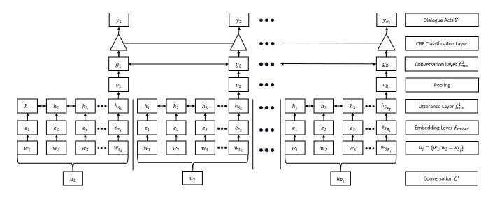
Figure 1: An illustration of our proposed hierarchical Bi-LSTM CRF model. The input is a conversation  $C^i$  consisting of  $R_i$  utterances  $u_1, u_2, \ldots u_{R_i}$ , with each utterance  $u_j$  itself being a sequence of words  $w_1, w_2, \ldots w_{S_j}$ . As can be seen, there are four main layers, viz. embedding, utterance encoder, conversation encoder, and CRF classifier. The output is a DA prediction for each utterance in the conversation.
