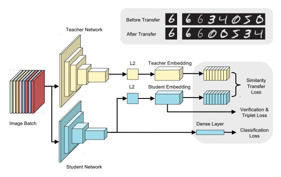
Figure 1: The network architecture of our DarkRank method. The student network is trained with standard classification loss, contrastive loss and triplet loss as well as the similarity transfer loss proposed by us.
