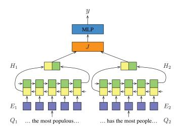
Figure 1: The structure of the BLSTM model.
