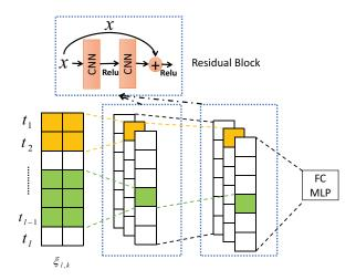
Figure 2: Our discriminator's structure follows a onedimensional CNN architecture in line with (Gulrajani et al. 2017). The input is l length sequence, where each element has k features. In the figure k = 2, while in our paper, k = 1, which is the inter-event time duration.
