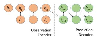
Figure 1: Our generator follows the sequence to sequence recurrent network in line with (Sutskever, Vinyals, and Le 2014). Different from the traditional MLE based learning loss, we update the seq2seq LSTM via a fused loss including both MLE and Wasserstein losses.
