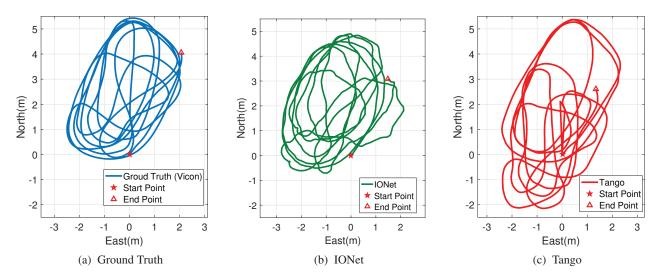
Figure 9: Trolley tracking trajectories of (a) Ground Truth (b) IONet (c) Tango
