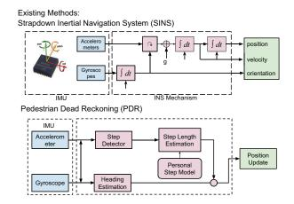
Figure 2: Architecture of existing methods: SINS and PDR
