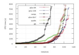
Figure 1: Cactus plot. A point at (x, y) means that the solver solved x instances each within y sec.
