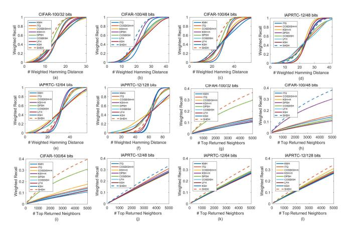
Figure 3: Weighted Recall curves on CIFAR-100 and IAPRTC-12. (a)  $\sim$  (f) show the Weighted Recall within various weighted Hamming distance at different number of bits. (g)  $\sim$  (l) show the Weighted Recall@n at different number of bits.
