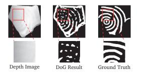
Figure 2: An illustration of using low-level methods for curve-structure segmentation. Serious erosion in the red square leads to very low contrast in the depth image, and low-level method, such as DoG (Difference of Gaussian), may produce very poor segmentation.
