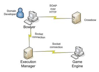
Figure 2: Components of the Zocalo Framework
