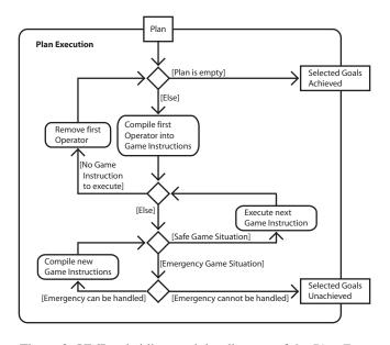
Figure 2: UML subsidiary activity diagram of the Plan Execution from Figure 1; it receives a plan as an input parameter and returns whether the plan's goals have been achieved. Operators from the plan are compiled, one at a time, into low-level game instructions such as path planning. These instructions are in turn executed one at a time, thus providing an opportunity to test for emergency game situations.
