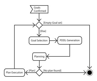
Figure 1: UML activity diagram of a PDDL-based Planning Component. Round rectangles represent subsidiary activities. The component begins with accepting the signal of goals confirmation and ends when this goal set is empty or else when no plan has been found. When the execution of a plan is a success, its goal are removed from the goal set by the subsidiary activity Plan Execution (see Figure 2).
