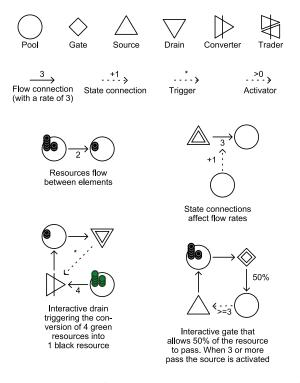
Figure 1: Elements of Machinations diagrams and example constructions.
