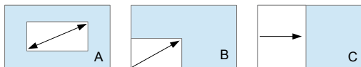
Figure 2: Reveal animations for RecognizePicture and rpMobile . Animations start from the center (A), a corner (B), or a side (C).
