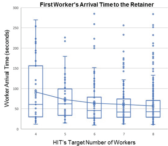
Figure 6: The distribution of the first workers’ arrival times when the system aimed to recruit various number of workers from mturk marketplace. A larger C_{market} results in not only a smaller mean of arrival time, but also a smaller standard deviation.
