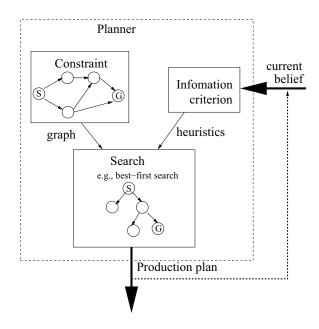
Figure 2: Planner for pervasive model adaptation
