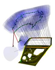
Figure 3: A solution of the task sequencing problem. The robot moves the laser scanner along the red path above the workpiece, and welds the seams from their access volumes, indicated by the blue truncated cones.
