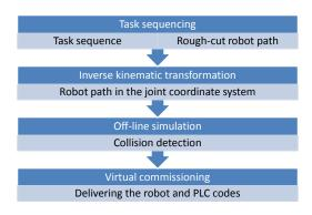
Figure 2: Workflow in the off-line programming system. The paper focuses on the first step, task sequencing integrated with rough-cut path planning.
