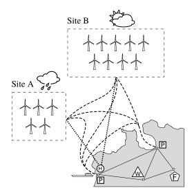
Figure 1: A typical wind-farm maintenance problem. Ships can sail along dashed routes, while helicopters can only leave from airports and move between wind-farms. Both ships and aircraft must Enter the site before being able to move amongst turbines, and Exit in order to return to port, making each wind-farm a restricted portion of the statespace. Nodes are labelled as follows: H – heliport, P – seaport, W – warehouse, F – factory.
