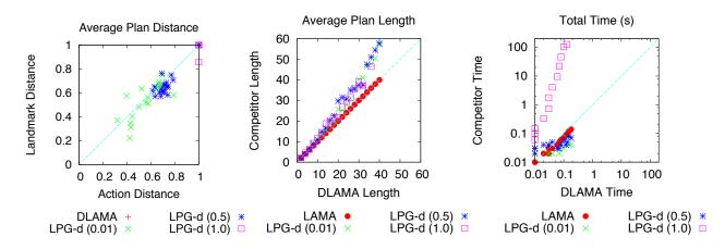
Figure 4: Average landmark-based and action set-based plan distance (left), average plan length (center), and total time in seconds (right) results on IN instances. The instances scale number of disjunctive landmarks from one to twenty.
