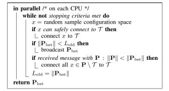
Figure 2: The C-FOREST Algorithm. The construction of  $\mathcal{T}$  depends on the planning algorithm being used (e.g, RRT\*). We assume asymptotically optimal convergence of  $\|\mathbf{P}_{bst}\|$ .
