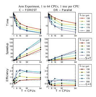
Figure 3: C-FOREST with SPRT vs. OR with SPRT for a 7 DOF arm. Color is target path length  $(L_{\text{target}})$ . Dashed lines show linear speedup ( $\eta = 1$  and S = T) with respect to CPUs. Time (mean, standard error), speedup, and efficiency using 1-64 CPUs, 1 tree per CPU (32 runs per data-point).
