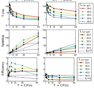
Figure 4: C-FOREST with SPRT vs. OR with SPRT, 4 robot team in an office. 32 runs per data-point. Same key as Fig 3.
