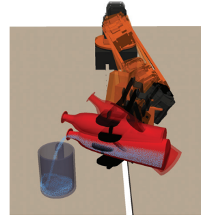
Figure 1: An example of a liquid transfer task performed by a 7-DOF ClamArm robot. We use an optimization-based planner that is tightly coupled with a fluid simulator and fluid transfer controller.
