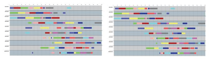
(a) Before post-optimization (TWT = 3347, NPE = 91.98 KWh) (b) After post-optimization (TWT = 3347, NPE = 31.35 KWh)
