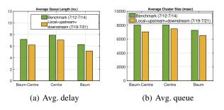
Figure 6: Initial field comparison on Baum-Centre corridors - average queue length and cluster size during PM rush hour.
