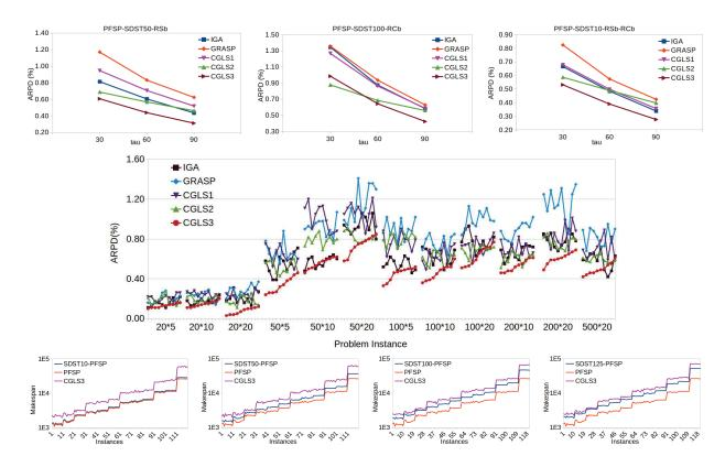
Figure 4: Top: Sample performance of the algorithms over different timeouts; Middle: ARPDs of 120 PFSP instances with SDST125 and RSb-RCb when  $\tau = 90$ ; Bottom: Comparison against lower bounds of makespan obtained from related problem.
