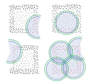
Figure 3: Placement ("+") and coverage points("x"). The footprint is the green circle. The footprint radius is reduced by  $\epsilon$  to the blue circle, ensuring that any gaps between the coverage points are covered by some green circle. Coverage points inside the blue circle are drawn in red and included in the MIP Q to model "if a footprint is placed here, these coverage points are covered." The optimal solution uses four footprints: two are centered outside the ROI.
