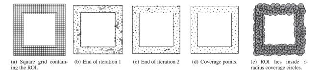
Figure 1: Creating *coverage* samples using  $\epsilon$  spacing. Coverage points are "x" and the small squares are the ones that are not yet covered by an  $\epsilon$ -radius circle centered at a coverage point.
