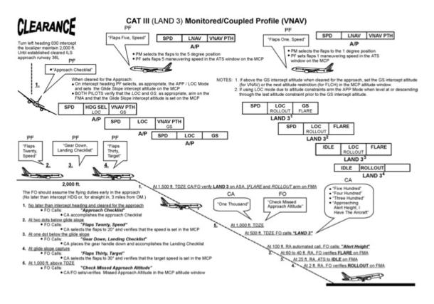
Figure 3: Procedure for flying an ILS CAT III approach from a Continental 777 flight manual
