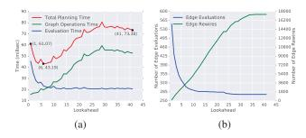
Figure 4: Computation times (a) and number of operations (b) of LRA\* as a function of the lookahead  $\alpha$ .
