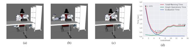
Figure 5: Manipulation experiments. (a-c) HERB is required to reach into the bookshelf while avoiding collision with the table. (d) Edge evaluation, rewiring and total planning time as a function of the lookahead.
