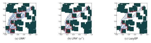
Figure 3: Visualization of edge evaluations by (a) LWA\*, (b) LRA\* with an optimal lookahead  $\alpha^*$ , and (c) LazySP. Source and target are (0.1, 0.1) and (0.9, 0.9), respectively. Edges evaluated to be in collision and free are marked red and blue, respectively.
