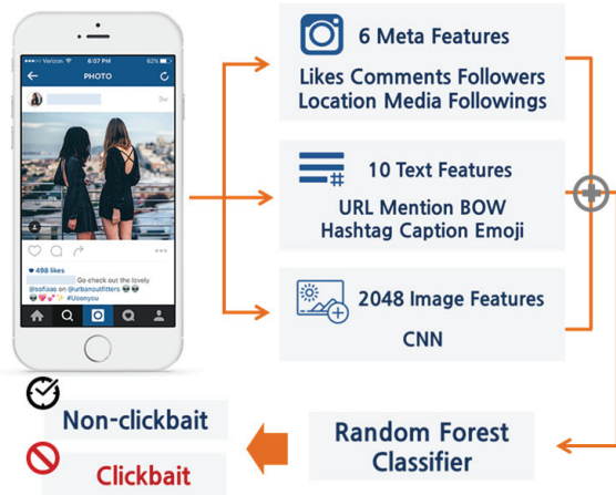
Figure 2: A diagram of the clickbait classification model applied to visual social media.
