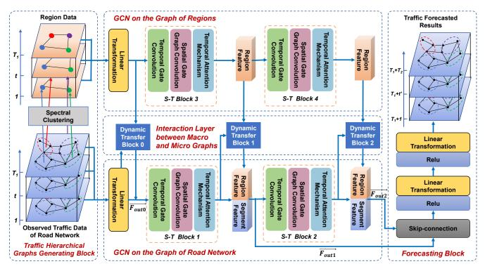
Figure 1: The proposed HGCN for traffic forecasting.
