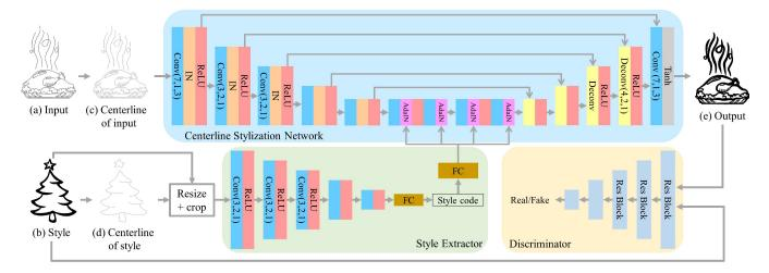
Figure 3: System overview. Our system formulates style transfer as an image-to-image translation where the centerline of the input is fed to a centerline stylization network and fused with the style code extracted from the style image via a style extractor. The fused features will be decoded to an output line image which is further justified by a discriminator.
