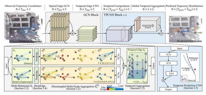
Figure 2: An overview of our DMRGCN model. Starting with 2-dimensional coordinates of N pedestrians for  $T_{obs}$  frames, we construct multi-relational graphs and then apply the disentangled multi-scale aggregation, followed by GCNs, on spatio-temporal pedestrian graphs. We then extrapolate future trajectories with TCNs and refine it with the GTA module.
