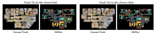
Figure 5: Object Navigation: Visualization of paths found by A\* using SMNet maps. Green and red squares indicate agent's starting and stopping locations. The grey color represents the floor pixels. The left example shows a case of success with high SPL = 0.8276 and the example on the right shows a case of success with low SPL= 0.4282.
