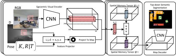
Figure 3: At each step in a trajectory, SMNet updates an allocentric map based on egocentric observations. Egocentric RGB-D observations are represented using a CNN encoder and the feature vectors are projected to the spatial memory (left). Memory cells are updated by a GRU to incorporate this new information (middle). The spatial memory can then be decoded by to perform top-down semantic segmentation (right).
