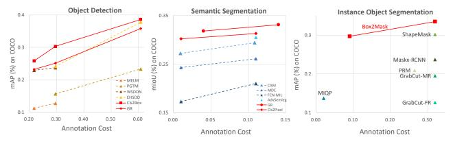
Figure 5: Comparative results on three sub-tasks with weakly/semi-supervised baselines under different annotation costs. We report the metrics on baselines with the same backbone. GR refers to the graph relation reasoning module.
