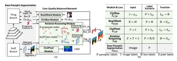
Figure 3: Illustration of the CQB-Net. Based on a panoptic segmentation network, we adopt four modules to unify different supervisions. (a) shows the Input/Output flow of the proposed modules. (b) summarizes the configurations of the four modules, including their input in (a), label scenario and function in terms of weakly-supervised learning.
