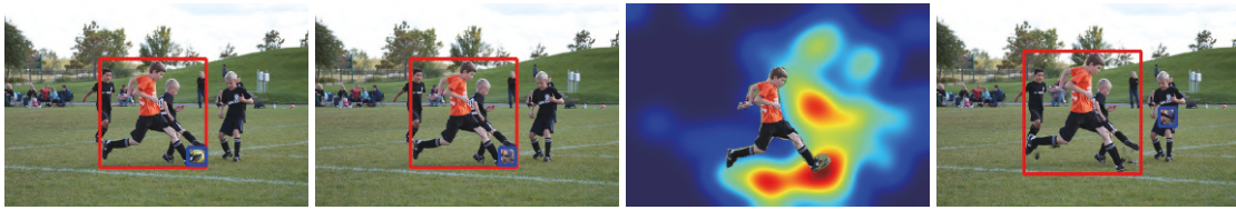
Figure 2: Overview of our method: the first image is the original input (red box: human, blue box: object). The second image is the result of local object appearance augmentation (Sec. ). The third and fourth images show the pose-guided probability distribution map and the result of global spatial correlation augmentation (Sec. ).
