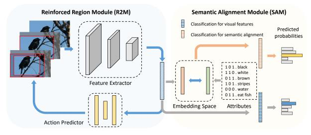
Figure 2: The framework of RL for GZSL (SR2E) model. SR2E achieves serialized search for discriminative regions using RL skills. R2M and SAM modules are included. R2M aims to localize the object region for more discriminative features. SAM focuses on facilitating semantic-visual alignment with a domain detector.
