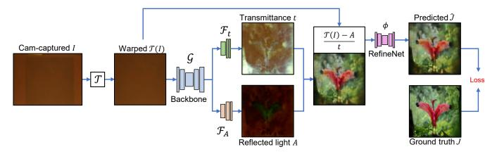
Figure 2: Network architecture of our Neural-STE. It consists of three modules: WarpingNet  $(\mathcal{G}, \mathcal{F}_A, \mathcal{F}_t)$  and RefineNet  $\phi$ . These modules together with the losses allow us to utilize our image formation model to effectively model privacy attacks on physical mail problem.
