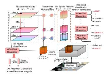
Figure 2: Structure of SSN. It takes an image as an input, and outputs N spatial features. Each pixel of X is estimated twice by the attention classifier
