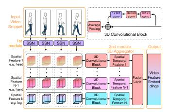
Figure 1: Overall Workflow of SSN3D. It takes a video snippet as input, and outputs a feature embedding vector
