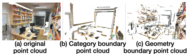
Figure 10: Three subsets of the point cloud used for the evaluation on indistinguishable points based metric. The background is colored white.
